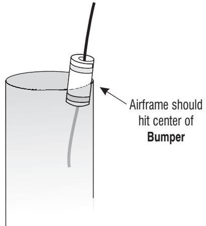
Once tied in place, roll the **Bumper** around itself and wrap the two strips of Velcro® around its body. Wrapping the bottom piece of Velcro® is a little bit difficult with smaller airframes but we’ve found that it can be done with less than a minute’s worth of labor.
